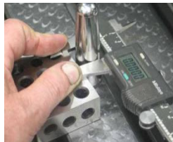
Fig.4 Measuring taper with the help of vernier calliper [Ref.12]
